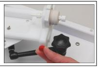
To switch the gray posts to accept an aorta section, loosen the red knobs and slide the post brackets off the ends of the rectangular support as shown. Turn the brackets around and slide them back onto the support, then tighten where you wish via the red knobs. Remove the luer lock caps from the ends of the posts and retain.
